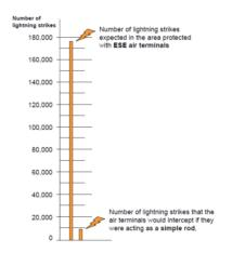
Fig. 7. Expected number of strike on the air-terminal
